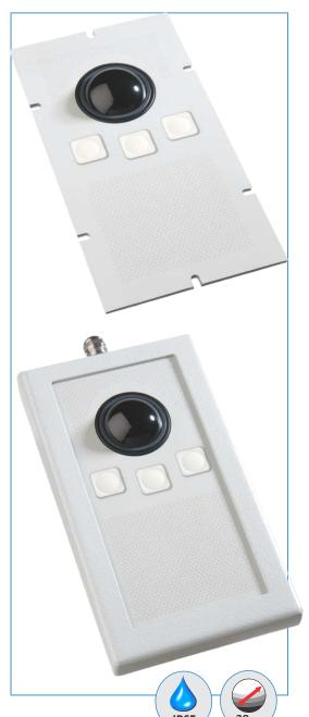
The TBM34 series is a ruggedised professional trackball. The unit has been specially designed for harsh industrial environment applications: the self-adjusting PTFE seal of the trackerball guarantees an IP65 static (ball in rest) protection grade. Carrier plates and housing are metal (aluminium and steel).
