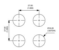
Rear mounted sealed pushbutton switches • bushing Ø 16 mm • metal • latching
