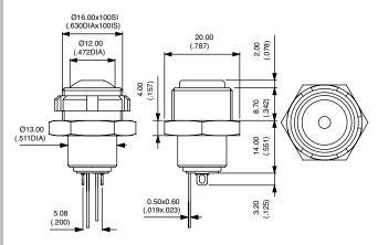
Rear mounted sealed pushbutton switches • bushing Ø 16 mm • metal • latching
